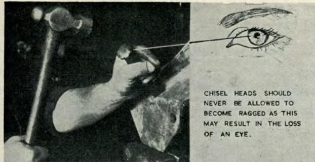
CHISEL HEADS SHOULD NEVER BE ALLOWED TO BECOME RAGGED AS THIS MAY RESULT IN THE LOSS OF AN EYE.
